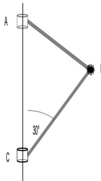
(c) The above diagram shows a mass of 10 kilograms at B connected by light rods (at right angles) to sleeves A and C which revolve freely about the vertical axis AC but do not move vertically. The angle between the vertical axis AC and the light rod BC is  $30^\circ$ . The acceleration due to gravity is  $9.8 \text{ m/sec}^2$ .
